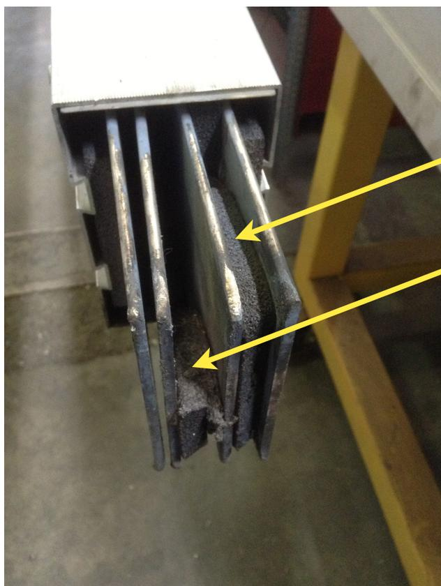
EX: the operator did not remove the insulation covers among the contacts... He joined the bars and turned on the current. As a result all fhe line witnessed a blast and the warranty on the product lost its validity.
